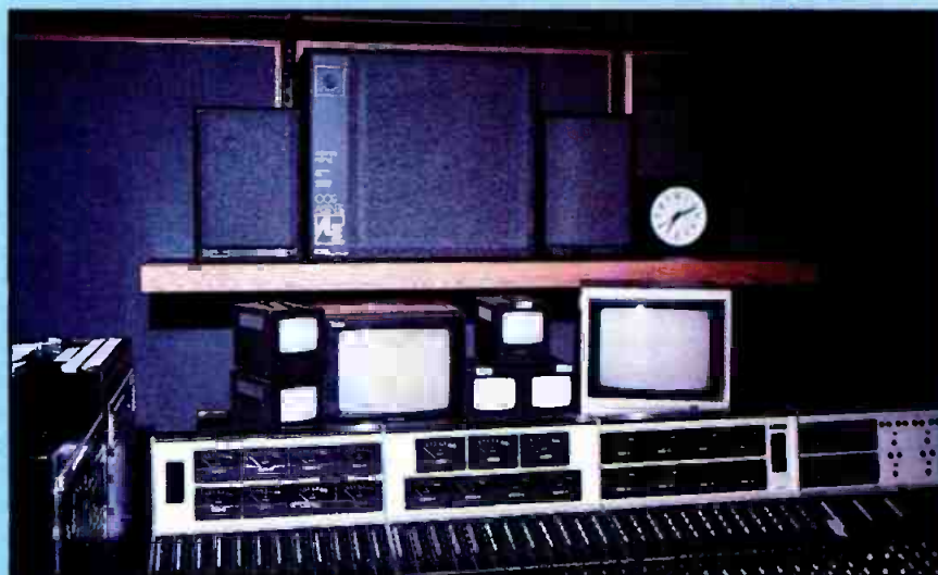
Mounted on a shelf above the Ward-Beck audio console is a pair of Sentry 100A loudspeakers and a larger size Sentry 500 between them.
